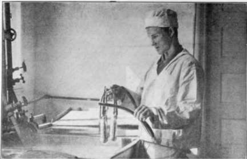
FIGURE 3.—The long milk tube with claw and teat cups is then detached from the head of the pail. Air tubes (on machines of inflation type) are plugged, and the whole is placed in a tank or a can of clean water, care being taken that all parts are entirely submerged.
